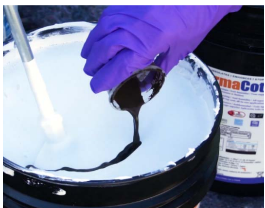
Procedure for mixing a pot of ThermoCote® with tinting
