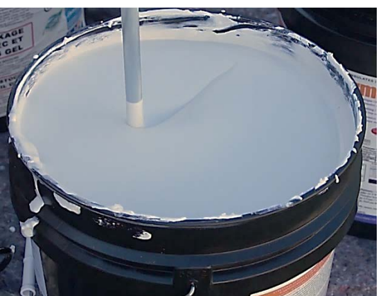
Procedure for mixing a pot of ThermoCote® with tinting
